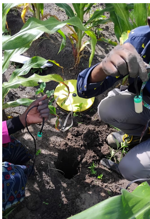
Installation of soil sensor
